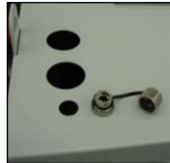
RJ-45 port on enclosure
